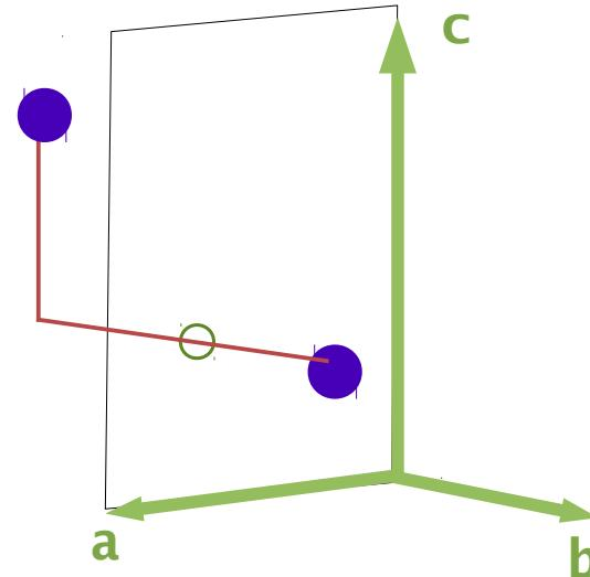
$$\begin{pmatrix} x \\ y \\ z \end{pmatrix} \xrightarrow{\text{red arrow}} \begin{pmatrix} x \\ -y \\ z + 1/2 \end{pmatrix}$$
